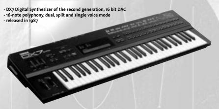
The 'new generation' of DX synthesizers (Mark-II) has 2-channel 6-operator 32-algorithm digital FM tone generators, which allows bi-timbral effects including stereo, splits and layers. Each of the two FM tone generators can be controlled independently via MIDI on separate channels, making the DX7 II FD do the work of two DX7s keyboards.
